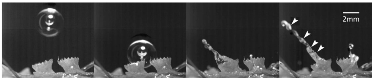
Fig. 2 Still frames from a video of a water drop hitting a gemmae cup of M. polymorpha off-center and transporting the gemmae-filled droplets. Filmed at 3000 fps with a 20 ms exposure. Arrows point to gemmae in the water droplets. The gravitational potential energy of the falling droplet is 1.4 \times 10^{-4} J. See Supplementary Video S1 .
